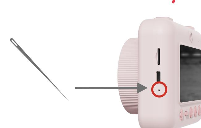
While the device is charging with the cable connected, locate a small hole on the side of the device. Use a paperclip or similar tool to press and hold the small button inside the hole for 30 seconds. You should feel a distinct click while pressing the button.
